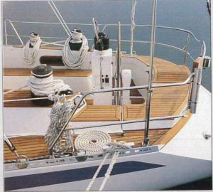
Turning lightly in two sets of ball bearings, the wheel conveys a precise feel of the helm. All important instruments and engine controls are close by, and the primary winches are near at hand and wholly visible. This is ideal for the cruising skipper.
