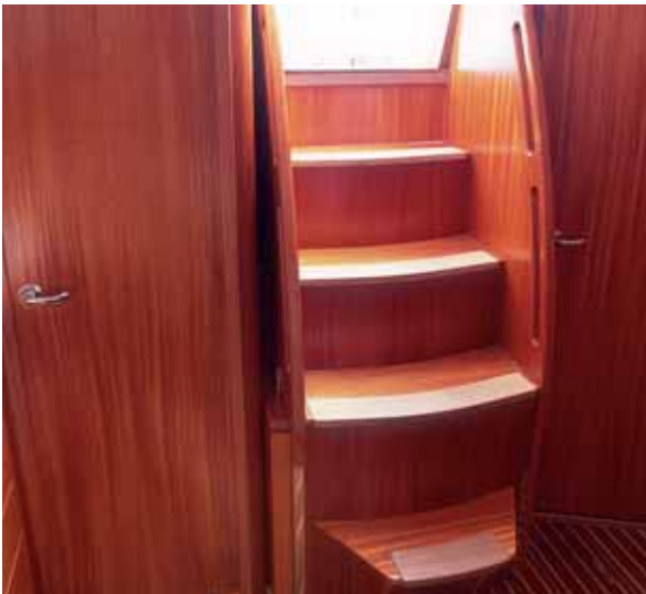
Gas strut operated staircase ...
